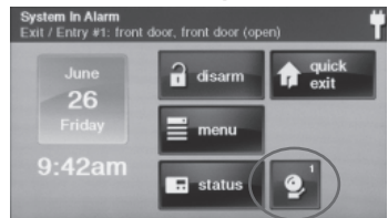
Security Screen with Alarm Memory Button
